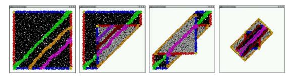
Figure 2: Folding an envelope structure, from [25]. A pattern of lines is constructed according to origami axioms. Elements then coordinate to fold the sheet using an actuation model based on epithelial cell morphogenesis.
