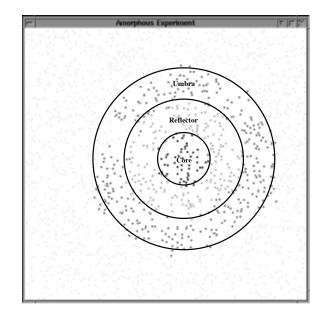
Figure 4: Anatomy of a Persistent Node. The innermost circle is the core (black), which arts as a virtual node. Every device within the middle circle is in the reflector (light grey), which calculates which direction the Persistent Node will move. The outermost circle (dark grey) is the umbra (k=3 in this example), which knows the identity of the Persistent Node, but nothing else.
