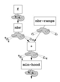
Figure 4: The **nbr** operation selects neighborhood values for computation at each point. Computing is carried out on neighborhoods with pointwise operations transformed to apply to neighborhood fields. Finally, a summary operation collapses each neighborhood of values into a single value for each point.
