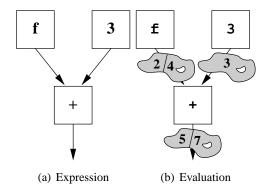
Figure 3: An expression is evaluated at a point in time by applying it to an amorphous medium, producing a set of fields as output. For example, the expression (+  $\bf f$  3) produces a field where every point mapped to n by  $\bf f$  maps to n+3 in the new field. General evaluation is instantaneous evaluation repeated at fixed intervals.
