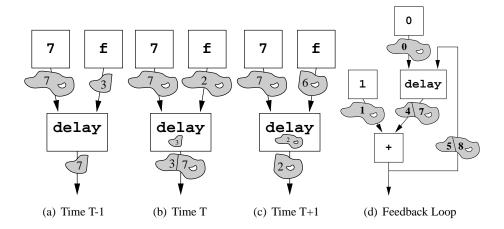
Figure 6: The **delay** operator, (**delay default input**), takes its scope from the current input and its values from the previous input, filling in any missing values with the initial value. The figure above shows three successive time-steps of the evaluation of (**delay 7 f**). The **delay** operator is used to create state variables using a feedback loop. For example, the counter shown in (d) starts at zero and increases by one each round.
