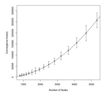
Figure 3: Convergence time scales quadratically as a function of network width. This plot shows a quadratic fit for number of nodes where width scales with number of nodes, holding expected number of neighbors fixed.
