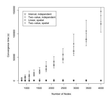
Figure 2: When initial values of devices are strongly correlated with a device's location in a spatial computer, convergence time scales much worse than when they are independent of position.
