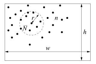
Figure 1: A spatial computer with unit disc communication and uniform random distribution of devices through a rectangular area can be described with five parameters: width w and height h, number of devices n, radius of communication r, and expected number of neighbors  $\bar{N}$ .
