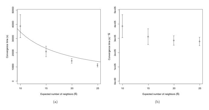
Figure 5: End-to-end convergence time (a) scales primarily with the inverse number of neighbors (inverse fit shown by line), plus a smaller factor from higher  $\bar{N}$  increasing the expected progress per hop and therefore decreasing diameter slightly. In (b) we plot  $\bar{N}$  against  $t \cdot \bar{N}$  to highlight the secondary effect from higher  $\bar{N}$ .
