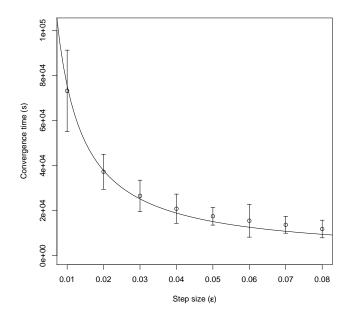
Figure 6: Convergence time is inverse linear with step size  $\epsilon$ , though this relationship breaks down as the system approaches instability. The line shown is an inverse linear fit, and the system is generally unstable for  $\epsilon > 0.08$ .
