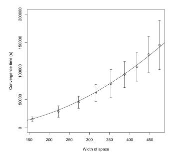
Figure 4: Convergence time depends on width, not number of devices. This plot shows a quadratic fit for width on simulations of n = 2000 devices in a fixed area with varying aspect ratio.
