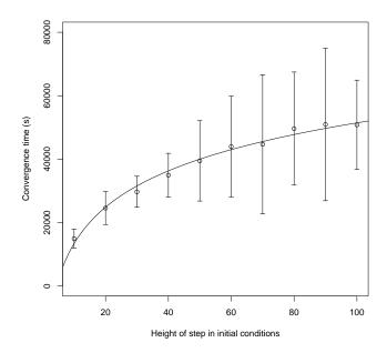
Figure 7: Convergence time scales logarithmically with the initial disagreement between nodes in the left and right halves of the distribution.
