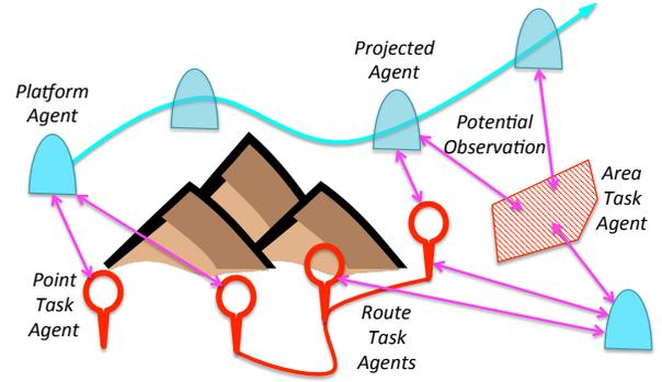
Fig. 3. In MTIP’s agent-based task allocation, agents for current platforms (light blue) and projections (translucent blue) along the platform’s anticipated trajectory communicate (purple arrows) with task agents (red) within line-of-sight and sensor range limitations to determine which tasks will be assigned to which platforms and on which segments of their anticipated route.
