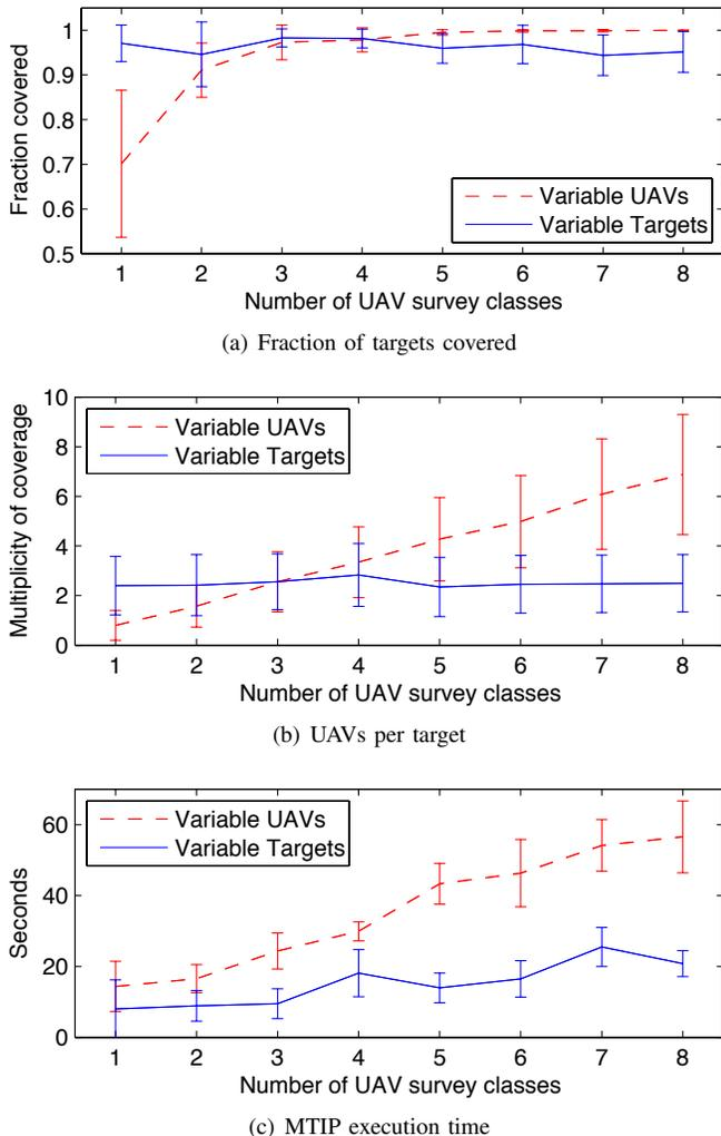
Fig. 8. Performance of MTIP sensor sharing with respect to variable numbers of UAVs ( $u$ ) or survey targets ( $t$ ): (a) even with few UAVs and many targets, the vast majority of targets are covered by at least one UAV, (b) most targets receive coverage from multiple UAVs, and (c) the time required for MTIP to make and dispatch allocation plans scales approximately linearly with both number of UAVs and number of targets. All graphs show mean over 10 trials  $\pm 1$  standard deviation.
