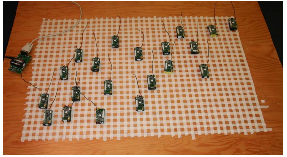
Figure 9: Our experimental network of 20 motes, laid out in a mesh-like network with synthetic coordinates. Reception range was software-limited to 9 inches, producing a 7-hop network. Data is gathered via the monitor device at the left.
